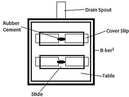
are shown here, but up to 6 can be accommodated per sample with this set up. A line drawing is included for clarification. Each B-ker<sup>2</sup> is 203 mm tall, with an inner square cross-section of 120 × 120 mm
