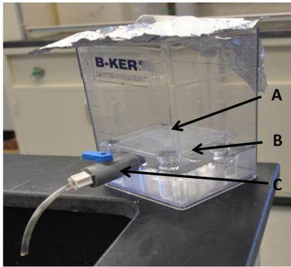
**Fig. 1** Settling chamber set-up. Coverslips (A) are set on slides which rest on a table (B) that sits above the level of the drain (C). The beaker is filled to the 2 L mark with water, and the sediment sample settles evenly over the surface of the table. Each coverslip represents a proportionate subsample. Four coverslips
